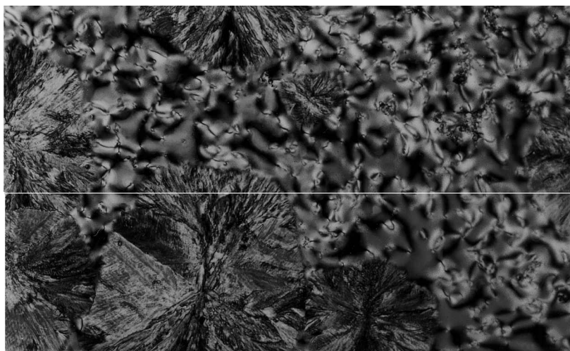
Figure. Optical textures of compound 3b obtained on cooling from the isotropic liquid at 185°C (crossed polarizers, magnification \times 100 ).
